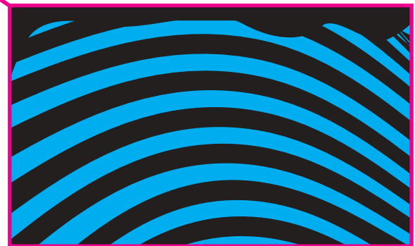
Spot UV varnish may peel off along the trim edge.
